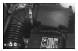
The engine air cleaner/filter is located on the driver's side of the engine compartment near the battery.
